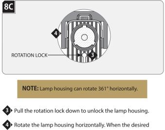
Rotate the lamp housing horizontally. When the desired position is achieved push the rotation lock up to lock the lamp housing in place.
