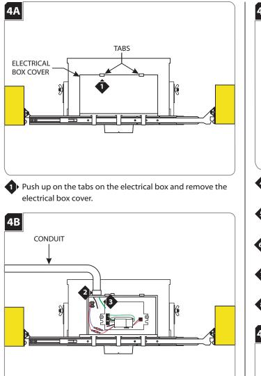
2 Install the conduit to the housing electrical box.
