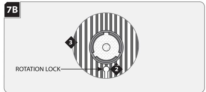
**NOTE:** Lamp housing can rotate 361° horizontally.
