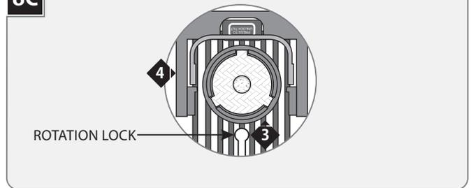
**NOTE:** Lamp housing can rotate 361° horizontally.
