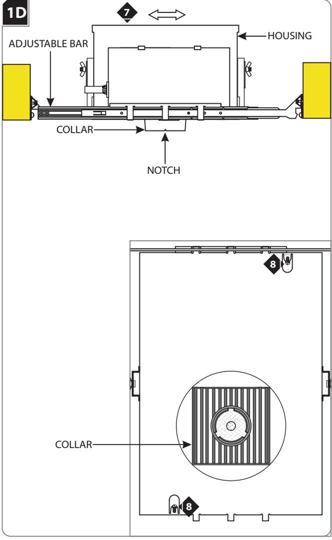
7 Adjust the collar position (horizontal position) by sliding the housing on adjustable bars.
