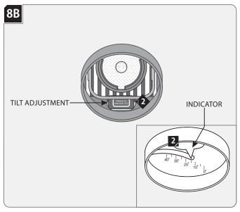
For proper wall wash positioning, unlock the tilt adjustment lever by pressing where indicated using a finger or screwdriver to tilt until 15° angle is reached.
