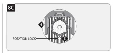
**NOTE:** Lamp housing can rotate 361° horizontally.
