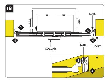
**NOTE:** The adjustable bars can be mounted to joists that are spaced 16" - 24" apart.
