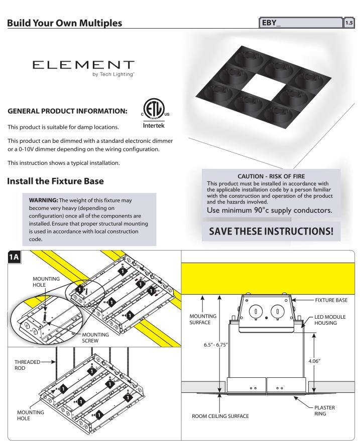
Use the 1/4" holes to suspend the fixture base with the use of threaded rods or use the screw holes to mount the fixture base securely in accordance with local construction code.
