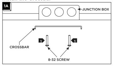
Mount the crossbar to the junction box with the provided #8-32 screws.
