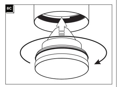
Install the reflector by inserting it into the bottom of the Cylinder and screw it in as far as it will go.
