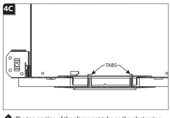
The top portion of the alignment tabs on the plaster ring should be broken off to avoid interference with the light module. Bend the tabs back and forth inside the housing to break the tabs.
