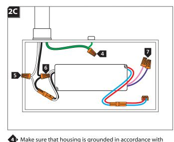
Make sure that housing is grounded in accordance with local electrical codes.
