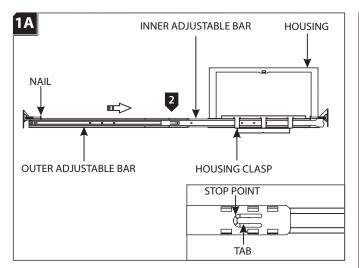
Remove the plaster ring from the housing. For flangeless trims, save the ring for step 4A. For flanged trims, the plaster ring can be discarded.
