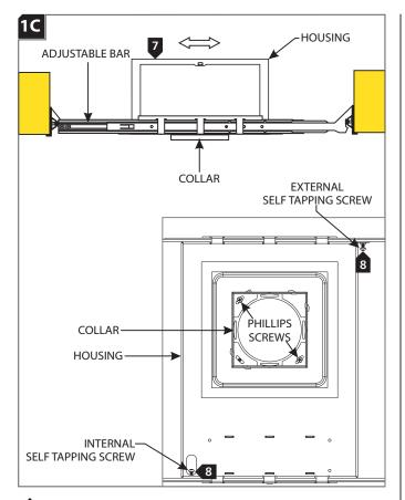
Adjust the collar's position (horizontal position) by sliding the housing on adjustable bars.
