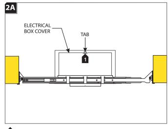
1 Push the tab on the housing electrical box up and remove the electrical box cover.
