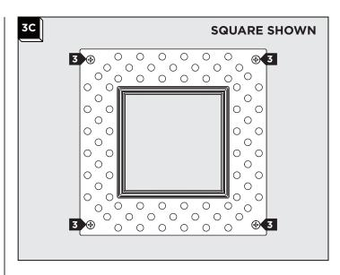
Secure the plaster ring by screwing the #8 screws (1" length) screws into the anchors.
