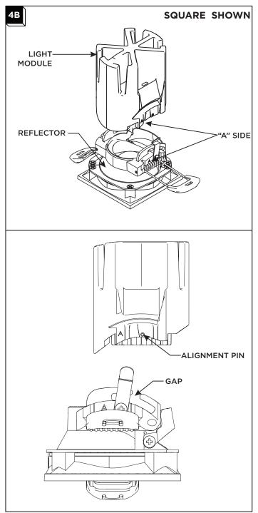
Carefully snap the light module and reflector together. On the adjustable versions, make sure to align the "A" sides and "B" sides of the two parts. Also, make sure the alignment pin on the light module passes through the gap in the mounting groove on the reflector.
