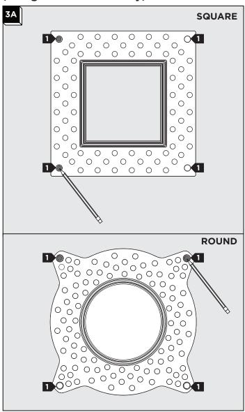
Mark the location of the four mounting holes, located in the corners of the plaster ring.
