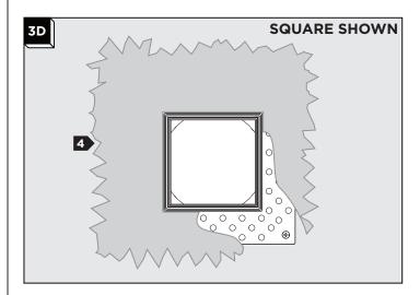
4 Properly plaster onto the plaster ring and drywall.
