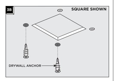
2 Install the four drywall anchors in the marked locations.
