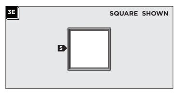
**5** Finish around the fixture to match drywall.
