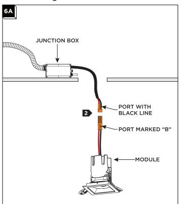
Connect the jumper cable to the housing wire making sure the port marked "B" is paired with the port with a black line.
