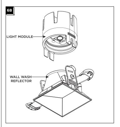
2 Snap light module and wall wash reflector together
