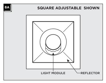
Using your fingers, adjust the direction of the light making sure to turn the module not the reflector (see note below).
