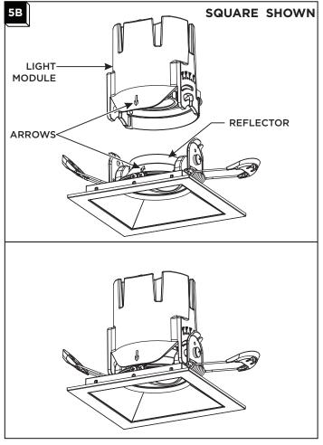
2 Carefully snap light module and reflector together. Alignment arrows are provided on the adjustable versions. Directional alignment is not required for fixed Versions.
