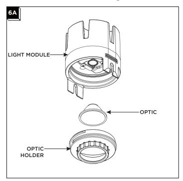
Remove and discard optic holder and optic from fixed light module.
