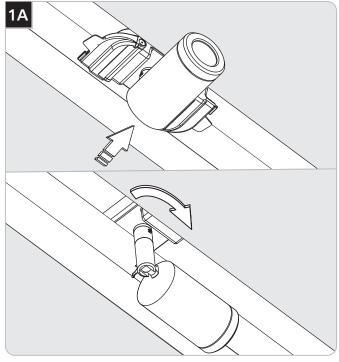
Install the capsule into the fixture channel at the desired location and rotate it 90° into place.
