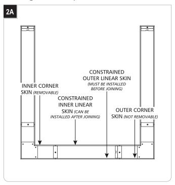
The previous instructions suggest connecting the units together with the side skins removed for ease of access. If installing 2 or more corners in a run, where linear units will be constrained at both ends by corners, please note the following:
