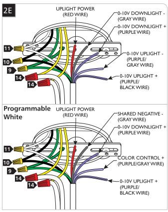
Connect the crossbar and the fixture ground wire to a suitable ground in accordance with local electrical codes
