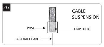
For cable suspension only: feed the aircraft cable through the post so that the grip lock is secured inside.
