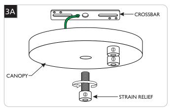
Remove the crossbar from the canopy and separate it from the threaded nipple by completely unscrewing it out.
