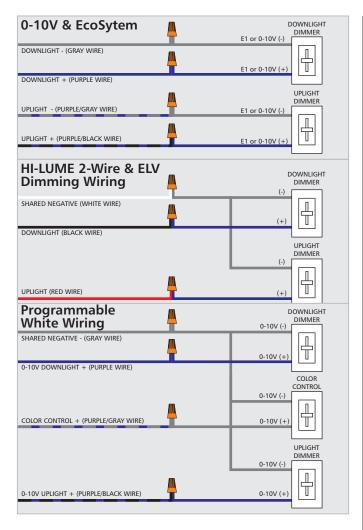
15 Connect the dimming wires as shown.
