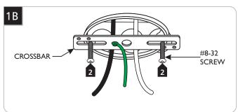
2 Mount the crossbar assembly to the electrical box with the two provided #8-32 screws.
