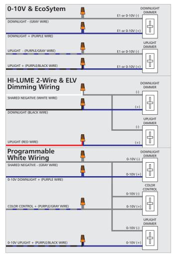
13 Connect the dimming wires as shown.
