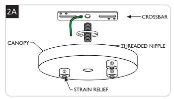
Remove the crossbar from the canopy and separate it from the threaded nipple by completely unscrewing it out.
