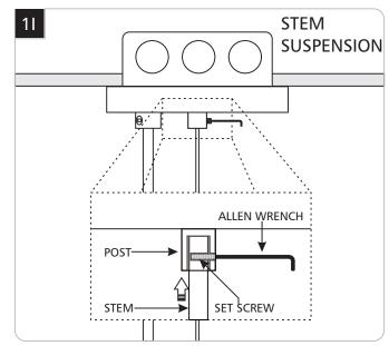
For stem suspension only: insert the stem into the post, align the stem hole with the post hole, and install the #6-32 set screw with the 1/16 Allen wrench. Make sure that the set screw is installed completely and tightly into the stem.
