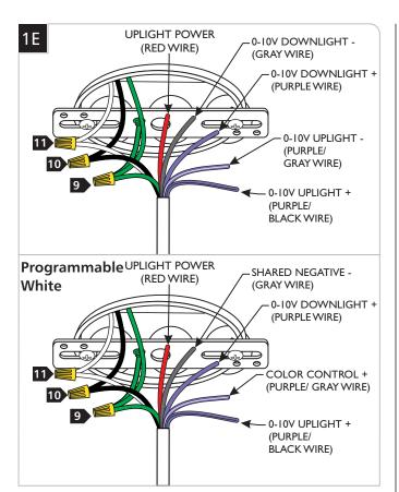
9 Connect the crossbar and the fixture ground wire to a suitable ground in accordance with local electrical codes.
