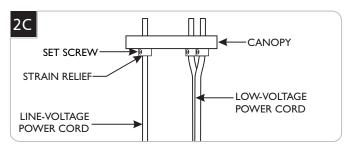
**NOTE:** The power cord does not support the fixture. For a casual "lazy cord" look, cut the power cord several inches longer than the drop height of the fixture.
