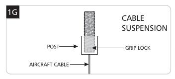
16 For cable suspension only: feed the aircraft cable through the post so that the grip lock is secured inside.
