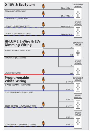
14 Connect the dimming wires as shown.
