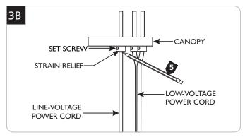
**NOTE:** The power cord does not support the fixture. For a casual "lazy cord" look, cut the power cord several inches longer than the drop height of the fixture.
