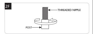
16 Screw the cable/stem post tightly onto the threaded nipple.
