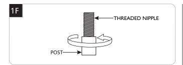
Screw the cable/stem post tightly onto the threaded nipple.
