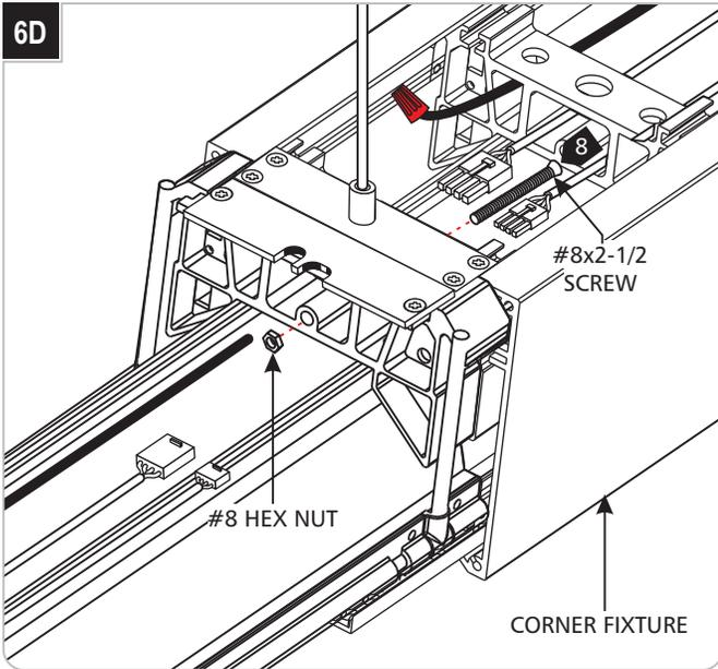
**8** Remove the top skins from the corner fixture. Install a 2-1/2" screw at each fixture joint. One screw will thread into the bracket in the adjoining fixture. The other will need the #8 hex nut provided. Use the hex wrench provided to pull the fixtures together and minimize the seam between the reflectors when seen from below. Raise or lower the ends of the fixtures as needed to align them.
