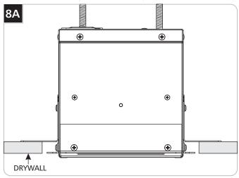
1 Install drywall up to the fixture housing(s).
