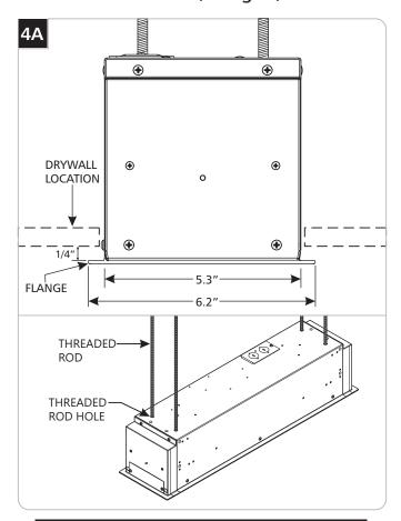
**NOTE:** If installing a continuous run, see section 6 for details before installation.
