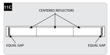
Slide the reflector(s) towards the center of the fixture/run so that there are equal gaps on each end.
