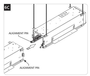
4 Using the alignment pins as a guide, slide the next fixture against the already installed fixture and secure the fixture in place using the preferred mounting method.
