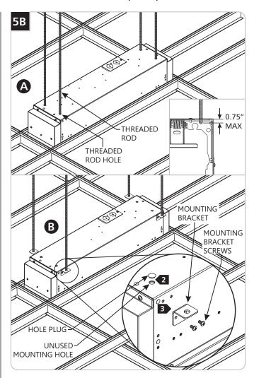
Choose one of the following installation options. If installing a continuous run, see section 6 for assembly details once an installation method has been determined. If not installing a continuous run, skip to section 7 once installation is complete:
