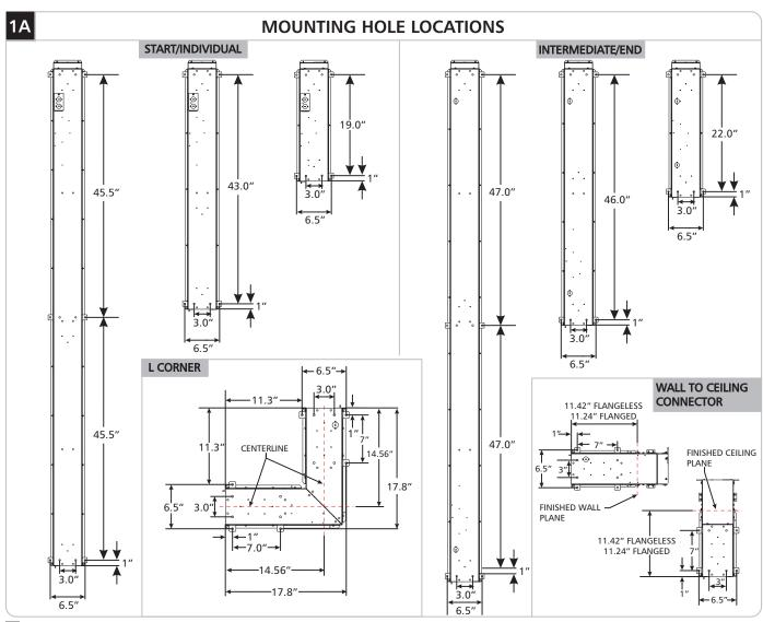
Install threaded rod or tie wire using the provided diagram for each model in the configuration.
