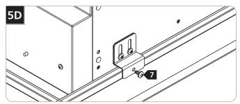
To further secure the fixture or per local code, use the screws slots on the sides of the brackets to secure the fixture to the T-bar.
