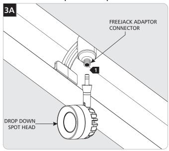
1 Screw the drop down spot head into the FreeJack female connector.
