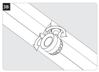
Tilt and/or rotate the spot head to the desired location.
