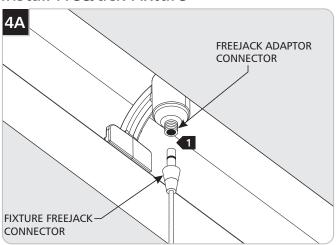
1 Screw the Fixture FreeJack male connector into the FreeJack female connector.
