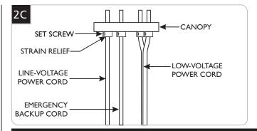
NOTE: The power cord does not support the fixture. For a casual "lazy cord" look, cut the power cord several inches longer than the drop height of the fixture.
