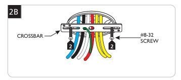
2 Mount the crossbar assembly to the electrical box with the two provided #8-32 screws.
