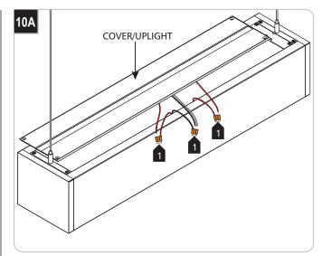
Connect the wires in the top cover to the corresponding wires inside the fixture using the push-in connectors provided.
