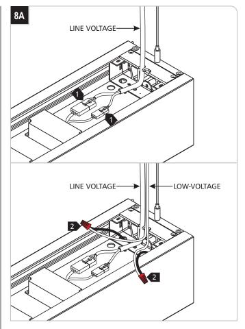
Connect the power and control wire connectors from the power feed to the connectors on the fixture.
