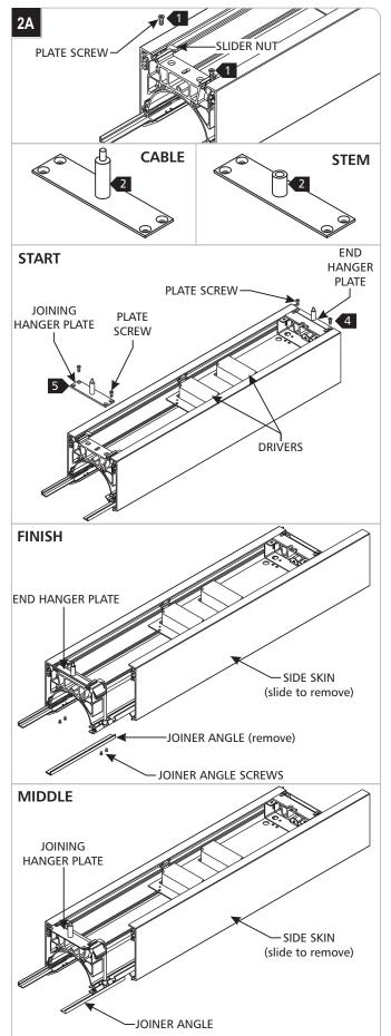
Note the plate screws mounted at each end of the fixture. These will be used to mount the hanging plates to the slider nuts.
