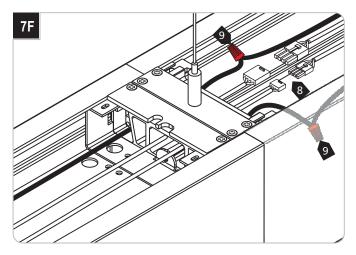
Feed the female power and control connectors into the adjacent fixture and connect them to the male connectors.
