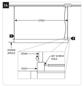
Temporarily install the fixture by pushing the stems completely into the posts and mark the location of the set screw hole. Make sure the joiner angles are facing the next connecting end.
