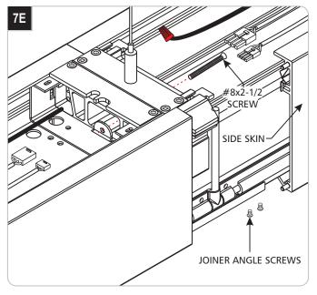
Install a 2-1/2" screw at each fixture joint. Use the hex wrench provided to tighten the screw and pull the fixtures together and minimize the seam between the reflectors when seen from below. Raise or lower the ends of the fixtures as needed to align them.
