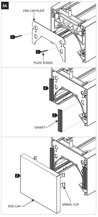
Remove the black gaskets from the end where present. Secure the end cap plate to both fixture ends using the provided plate screws.
