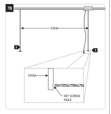
2 Remove the fixture and drill a hole using a #29 (0.136") drill bit at the marked location in each stem.
