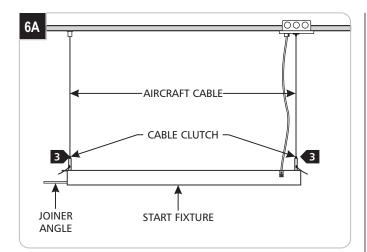
• Feed the aircraft cable completely through the cable clutches on the start fixture until the desired height is achieved. Make sure the joiner angles are facing the next fixture.
