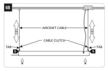
**2** To level the fixture, push the tab on the cable clutch and feed more or less of the support cable into the cable clutch. Make fine adjustments to each cable until the fixture is level.
