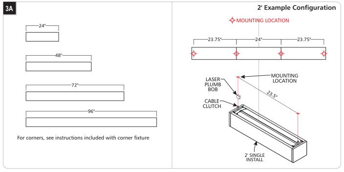
The mounting cable/stem locations on the fixture are centered at the seam between adjoining fixtures. The mounting location for the start and end fixtures are 1/4" in from the end. If installing a single fixture, mounting locations will be a 1/4" in from both ends. Using the provided diagram, mark the post/T-Bar location on the ceiling/grids for each model in the configuration. See example configuration.
