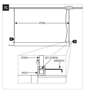
Reinstall the fixture by inserting the stems into the posts and install the #6-32 set screw with the 1/16 Allen wrench. Make sure that the set screw is installed completely and tightly into the stem.
