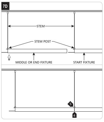
4 Set the free end of the new fixture onto the previous fixture's joiner angles. Push the fixtures together so that they are aligned and the reflectors are touching. Be careful not to dislodge the light leak gaskets or pinch them between the reflectors.
