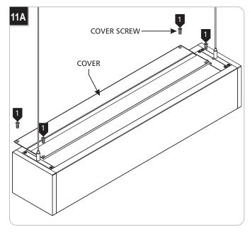
Neatly tuck in any wiring and secure the cover to the top of the fixture using the provided cover screws.
