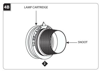
Unscrew the snoot from the lamp cartridge.
