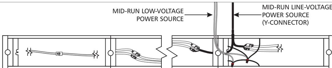
The line-voltage power can be delivered mid-run by using the Y-connector to connect the line-voltage and dimming controls. The low-voltage power can be delivered mid-run by connecting the low-voltage wires from the 2 adjacent units to the wire from the drop.
