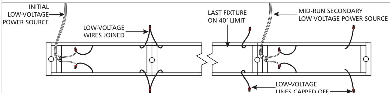
The low-voltage section of the fixture run will also likely be powered at the start of the run, then interconnected to a maximum of 40'. Sections of the run may be isolated by simply not connecting the low-voltage lines and the run may be powered by multiple transformers at different units to power longer runs.
