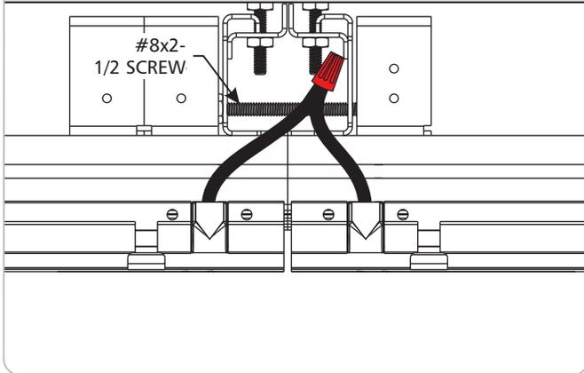
**7** Install a 2-1/2" screw at each fixture joint. Use the hex wrench provided to tighten the screw and pull the fixtures together and minimize the seam between the reflectors when seen from below.
