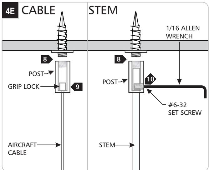
**8** Screw the posts onto the threaded washers.
