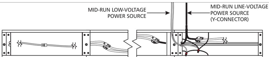
The line-voltage power can be delivered mid-run by using the Y-connector to connect the line-voltage and dimming controls. The low-voltage power can be delivered mid-run by connecting the low-voltage wires from the 2 adjacent units to the wire from the drop.
