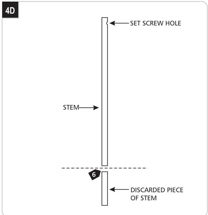
**5** If shortening the stems: starting from the end with the set screw hole, measure then mark the desired length of the stem.
