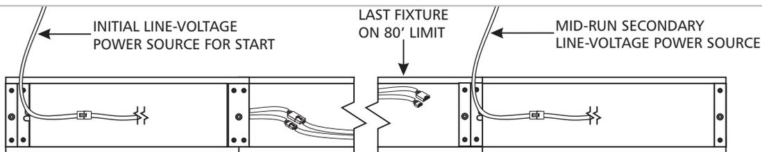
The line-voltage section of the fixture run will be likely powered at the start of the run, then interconnected to a maximum of 80'. For a longer run, sections may be isolated by simply not connecting the wire harnesses together. The secondary power source must be spliced to the wiring harness in the fixture using one of the provided notched locations.
