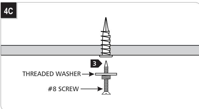
**3** Mount the threaded washer to the anchor with the #8 screw.
