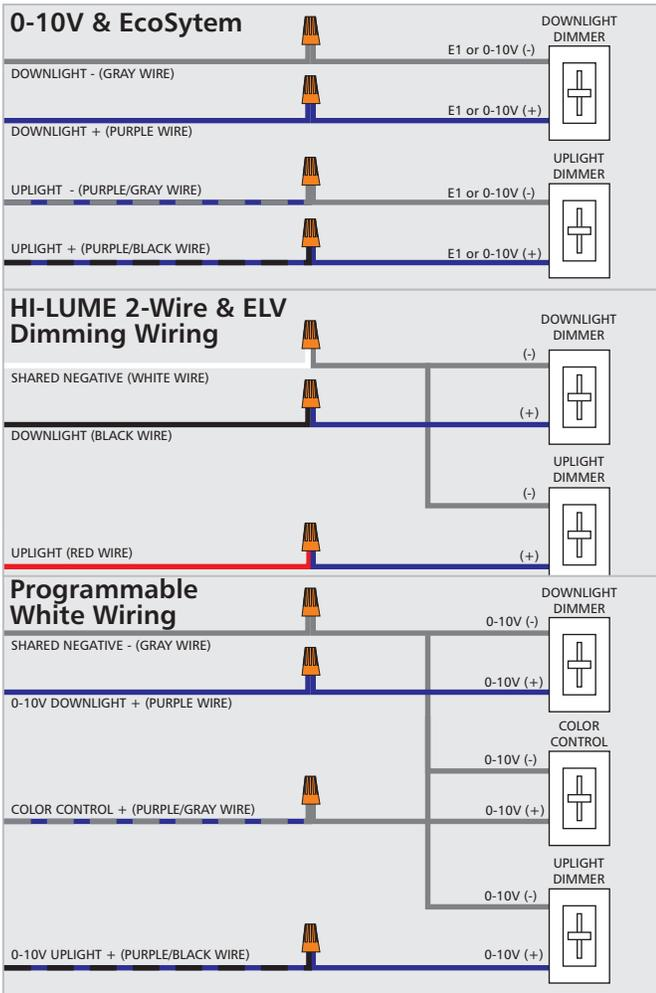
14 Connect the dimming wires as shown.
