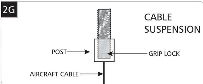
17 For cable suspension only: feed the aircraft cable through the post so that the grip lock is secured inside.
