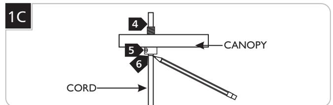
**3** With the planned height of the fixture in mind, feed the power cord through the strain relief until the desired look is achieved.
