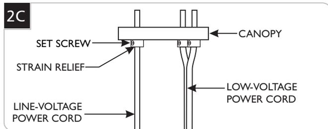
**NOTE:** The power cord does not support the fixture. For a casual "lazy cord" look, cut the power cord several inches longer than the drop height of the fixture.
