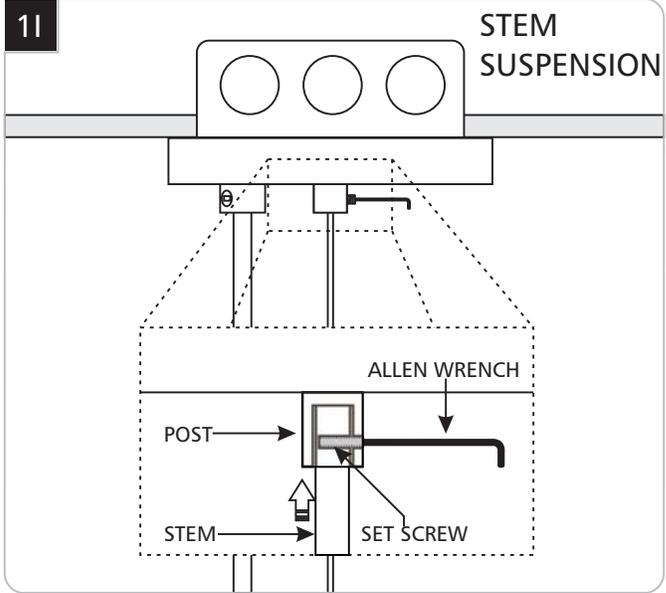
**20** For stem suspension only: insert the stem into the post, align the stem hole with the post hole, and install the #6-32 set screw with the 1/16 Allen wrench. Make sure that the set screw is installed completely and tightly into the stem.
