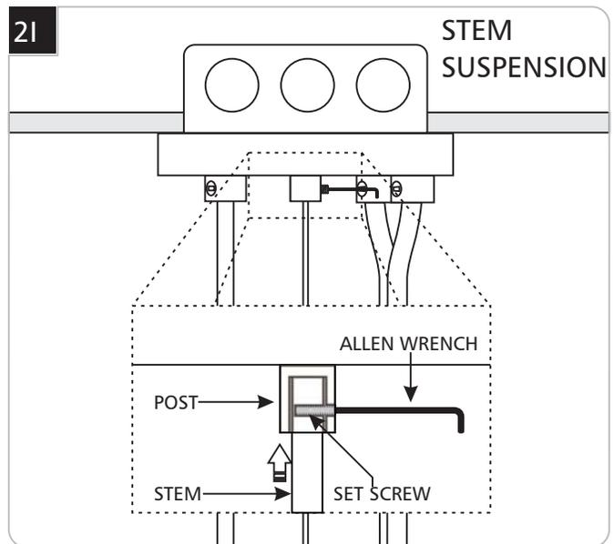
21 For stem suspension only: insert the stem into the post, align the stem hole with the post hole, and install the #6-32 set screw with the 1/16 Allen wrench. Make sure that the set screw is installed completely and tightly into the stem.
