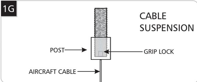
**16** For cable suspension only: feed the aircraft cable through the post so that the grip lock is secured inside.
