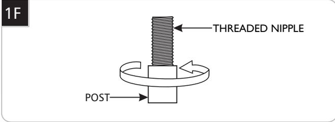
**15** Screw the cable/stem post tightly onto the threaded nipple.
