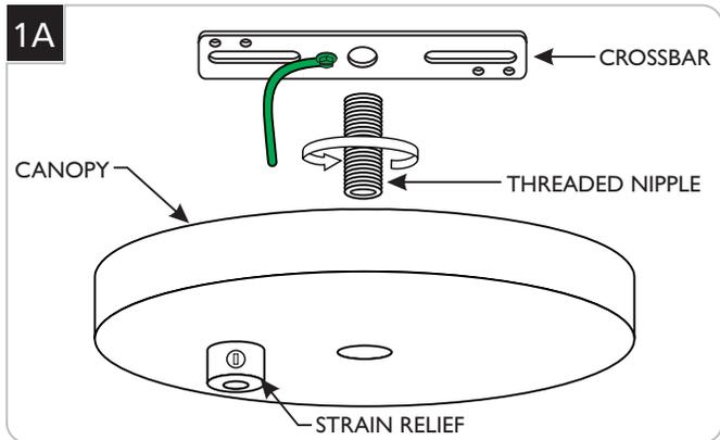
**1** Remove the crossbar from the canopy and separate it from the threaded nipple by completely unscrewing it out.
